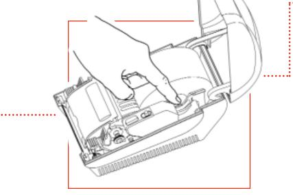
With the media roll loaded, press the green guide lock for easier media installation next time.
